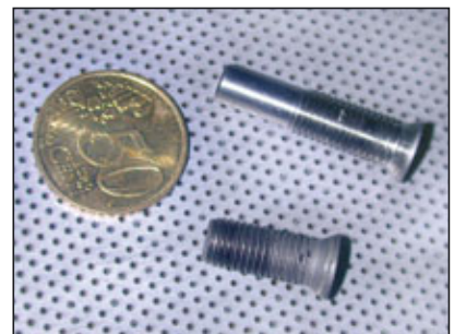
Changing balance screws on a CFM 56 engine (images courtesy of Deutsche BA)
