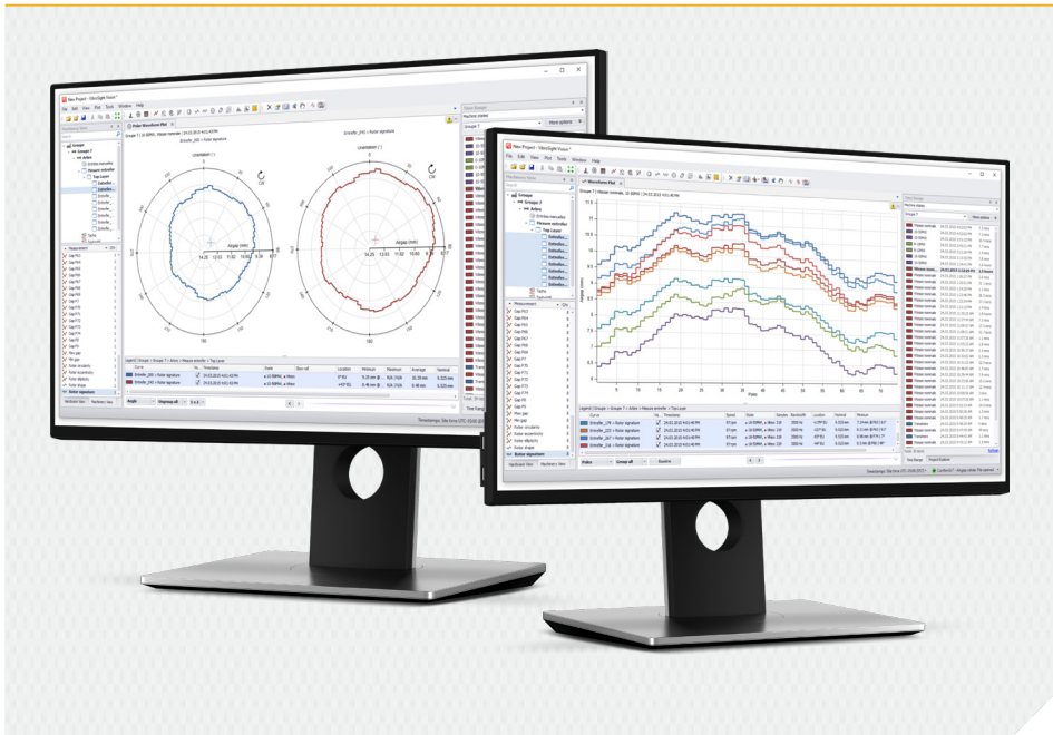
Figure 6: The VibroSmart and VM600 platforms are fully supported by VibroSight software including the diagnostic rule box "decision support" capabilities (top) and the specialized plot types such as air gap (bottom) unique to hydro machines.
