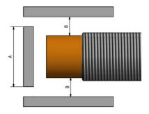
A = Target object diameter: ≥27 mm.
