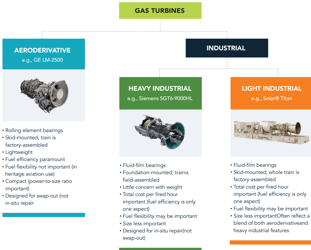
Figure 6: When used for mechanical drive, power generation, and marine propulsion, gas turbines can be broadly classified into the three categories shown here. The high-level attributes listed convey some of the key distinctions that help distinguish each category.
