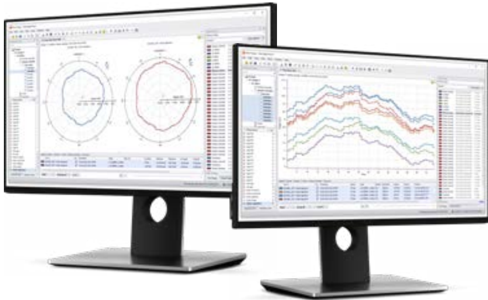
Figure 6: The VibroSmart and VM600 platforms are fully supported by VibroSight software including the diagnostic rule box “decision support” capabilities (top) and the specialized plot types such as air gap (bottom) unique to hydro machines.
