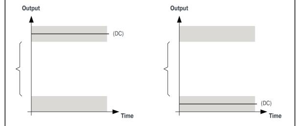
(b) Quasi-static (DC) component value = outside of the GSI127's normal operating range. A quasi-static (DC) component value outside of the GSI127's normal operating range is a diagnostic value, used to indicate that the GSI127 has detected a problem and that the measurement chain is not OK!
