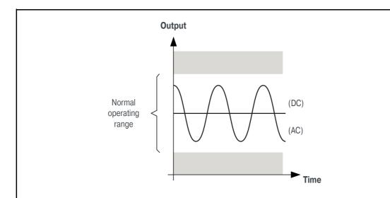
(a) Quasi-static (DC) component value = inside of the GSI127's normal operating range. A quasi-static (DC) component value inside of the GSI127's normal operating range is a non-diagnostic value, so the measurement chain is OK and both measurement components (AC and DC) of the output signal can be trusted and used.
