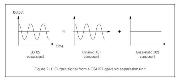
For the output signal from a GSI127 galvanic separation unit:
