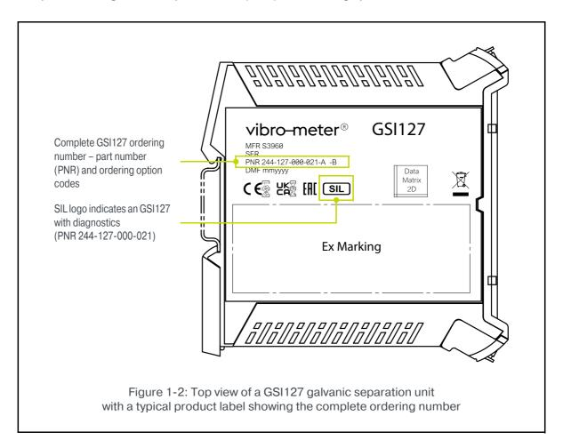
NOTE: A GSI127 galvanic separation unit with diagnostics (PNR 244-127-000-021) suitable for use in safety-related applications is identified by a SIL logo.
