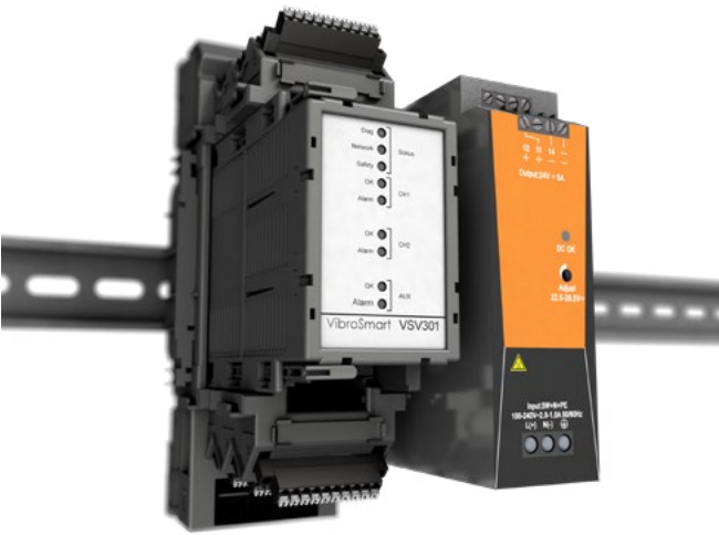
Figure 5: The simplicity of the VibroSmart system is evident in a system that requires only two module types: one for communications and one for universal signal processing applications (shown here) including the suite of measurements used for hydro machinery.
