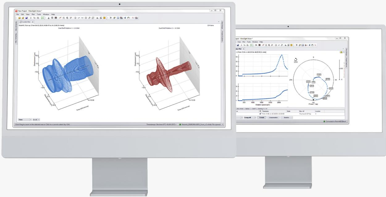
VibroSight provides the plot types – such as the Bode and Polar formats shown here – that are familiar to users of critical rotating machinery. However, it also provides dozens of other plot types and visualization capabilities that make it suitable for all classes of machinery.
