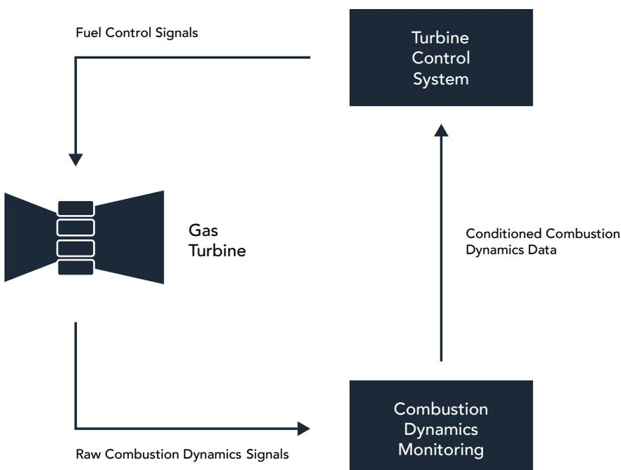
Combustion dynamics monitoring is part of closed-loop control to ensure that damaging pulsations in low-NO<sub>x</sub> gas turbines do not prematurely age or destroy the combustor cans. The pulsations occur because today's low-NO<sub>x</sub> technologies rely on inherently metastable combustion conditions that burn fuel in the leanest possible manner but can produce an unstable flame if not meticulously controlled.
