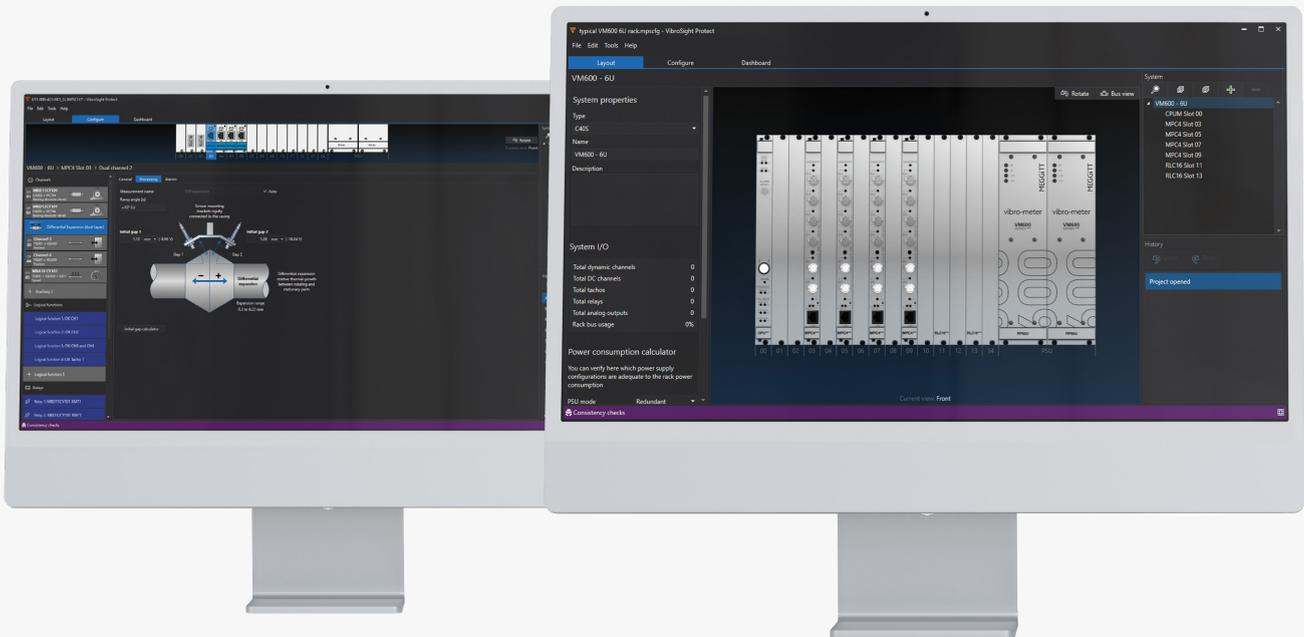
The VM600's all-new configuration environment is integrated in our VibroSight suite of software. It is called VibroSight Protect and relies heavily on graphical – rather than text-based – input for most configuration settings. Drag-and-drop, copy-and-paste, and other time-saving capabilities are now available that eliminate tedious configuration tasks and reduce the time required to configure a rack by 50% or more.
