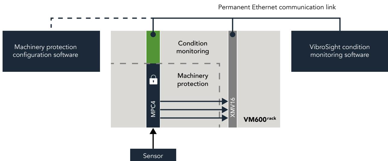
The new MPC4<sup>Mk2</sup> module provides integrated condition monitoring functionality identical to that of a separate XMV16 module, but in a manner that completely segregates the protective functions (black) from the condition monitoring functions (gray). Like its predecessor, the same sensors can be shared between protective and condition monitoring functions via the rack's backplane.
