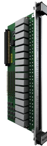
The relays on the RLC16<sup>Mk2</sup> module (shown) and the MPC4<sup>Mk2</sup> module (not shown) are now epoxy-sealed as well as being significantly easier to configure and wire.
