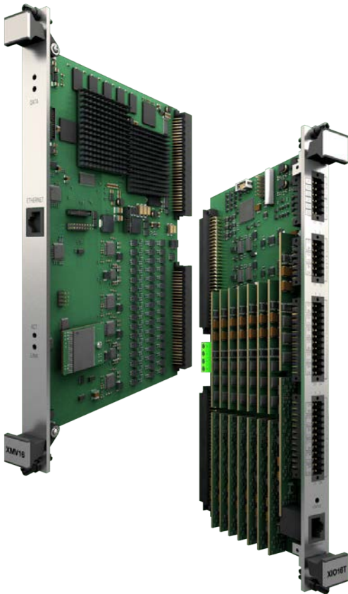
Figure 5: The VM600 XMV16 condition monitoring module consists of the signal processing and computation module (left) and the companion I/O module (right). It accepts a total of 16 dynamic signals from vibration and other sensors, and 4 tachometer signals used for speed or phase reference measurements. Gigabit Ethernet ports are provided on both the processing module and the I/O module; either one can be used to connect the processed data from the XMV16 to VibroSight condition monitoring software. The XMV16 can accept dynamic vibration signals from elsewhere in the VM600 rack via the system backplane, or (as in this project) via externally wired connections to the I/O module.
