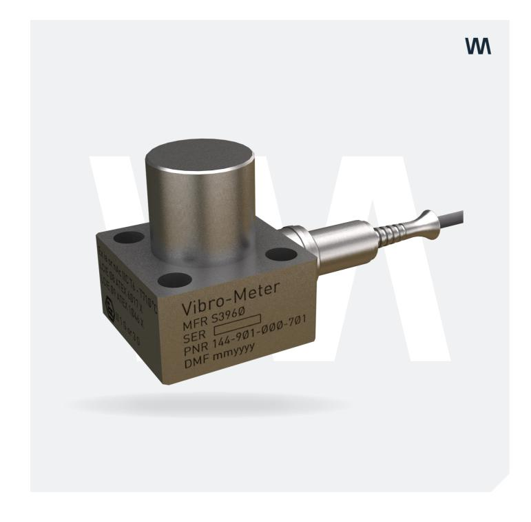
The CA series of vibration sensors are high-temperature, piezoelectric-based accelerometers designed for the long-term measurement and monitoring of absolute vibration in the most severe of environments.
