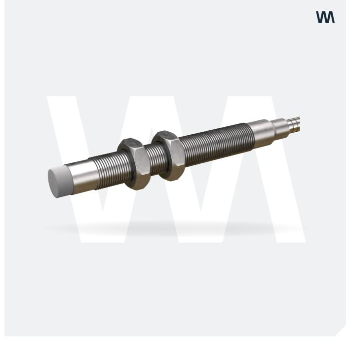
The WW and RE series of proximity sensors are used in combination with a transmitter or converter for direct 4 to 20 mA current measurement of shaft vibration or relative displacement. Measurements are made according to the eddy-current principle.
