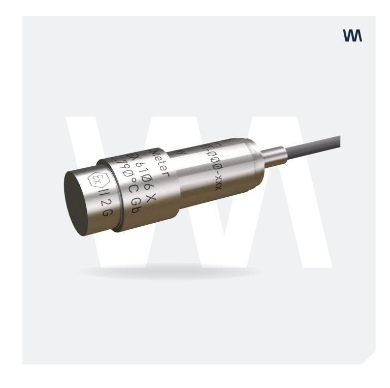
The CP series of dynamic pressure sensors are hightemperature, piezoelectric-based pressure sensors designed for the long-term measurement and monitoring of combustor pulsations and combustion dynamics in gas turbines.
