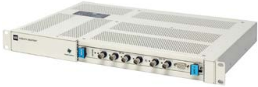
Figure 6: The VM600 "slimline" rack is just 1U tall and designed for mounting in a 19" cutout or on 19" EIA rails. It provides all necessary power and holds a single VM600 module such as the XMV16 shown here to provide a 20-channel condition monitoring solution (16 dynamic channels + 4 tachometer channels). The slimline chassis can also be used with other VM600 modules such as the MP-C4Mk2 to provide a compact, 4-channel machinery protection solution.
