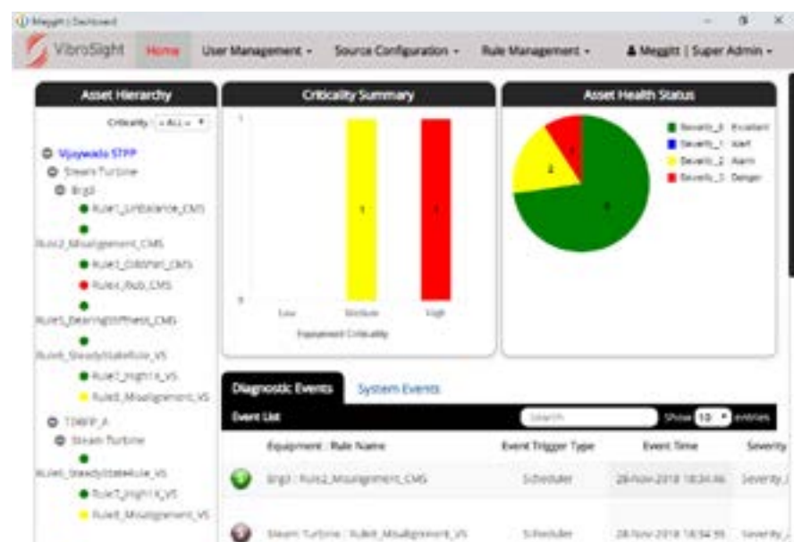
Figure 9: Many customers prefer the user interface of VibroSight's Rule Box software as the primary window into their condition monitoring system because it provides a high-level dashboard summarizing anything an operator needs to act on. Instead of complicated and specialized plots, it uses simple status indicators and narrative descriptions of problems detected, their severity, and what actions to take. This dashboard is taken from an actual vibro-meter installation at an STPP in India.
