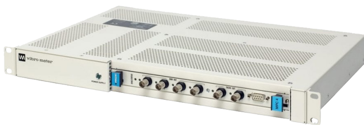
Figure 6: The VM600 "slimline" rack is just 1U tall and designed for mounting in a 19" cutout or on 19" EIA rails. It provides all necessary power and holds a single VM600 module such as the XMV16 shown here to provide a 20-channel condition monitoring solution (16 dynamic channels + 4 tachometer channels). The slimline chassis can also be used with other VM600 modules such as the MPC4 Mk2 to provide a compact, 4-channel machinery protection solution.
