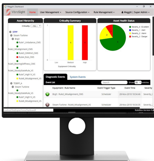
Figure 9: Rule Box allows automated malfunction diagnosis using rules that can be configured by vibro-meter or by the end-user using mathematical, logical, and other operators. The rule building environment is graphical and highly intuitive, as shown here, accomplished by simply joining operators. The result is rules that are powerful yet easy to build and easy to understand. Notice here that the selected output node at the top of the diagram (as noted by the blue "glow") has severity level 0 as indicated in the properties box. Complex rules can have multiple outputs that result in various severity levels.
