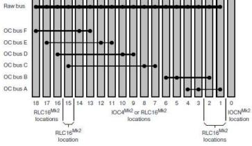
Restrictions according to the VM600 rack backplane OC bus connections
