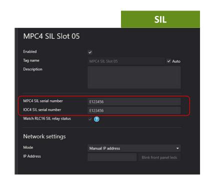
Verification of MPC4 and IOC4 serial numbers
