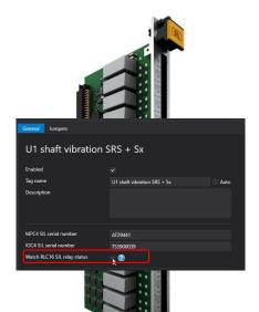
Raw bus is used for diagnostics and safety lines (force relays of RLC16 to go to "safe" output in case of problem)
