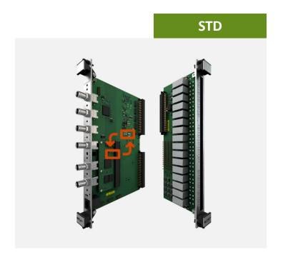
The replacement MPC4 it is autoconfigured by the IOC4
