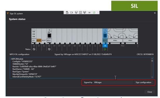
Protection configuration must be activated and then signed
