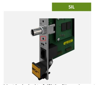
Must be locked to fulfil the SIL requirements
