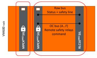
One SIL2 system is composed of MPC4 + IOC4 Mk2 SIL modules and 1 RLC16 Mk2 SIL module (optional)
