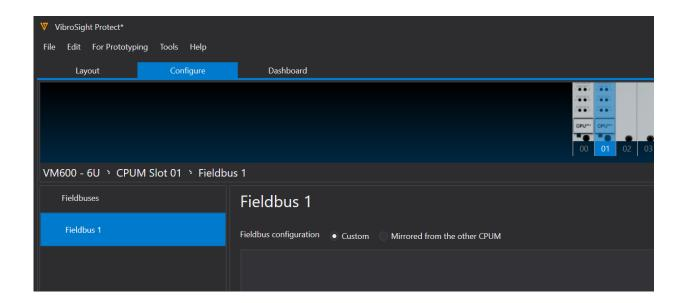
To maintain system integrity and prevent configuration conflicts, a consistency check has been implemented to restrict simultaneous configuration of both CPUMs as mirrored. This ensures that each CPUM operates independently or in a redundant configuration, contributing to enhanced system reliability and stability.
