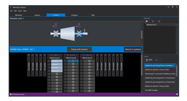
The XMV16 and XMVS16 cards offer 16 dynamic input channels and 4 speed input channels, providing users with extensive connectivity options for machine trains. These channels can be connected to the machine trains in the same manner as with MPC4<sup>Mk2</sup> cards, ensuring seamless integration into existing setups.
