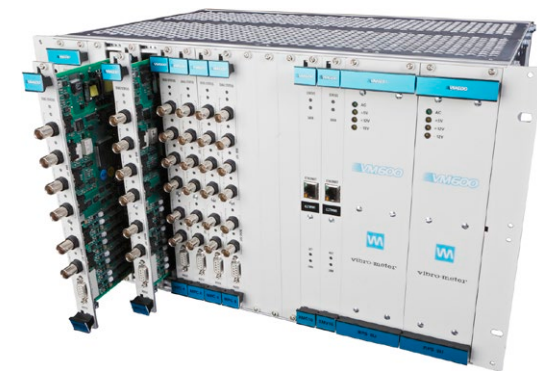
Photo of VM600 rack containing XMV16/XIO16T conditioning monitoring card pairs and MPC4/IOC4T machinery protection card pairs
