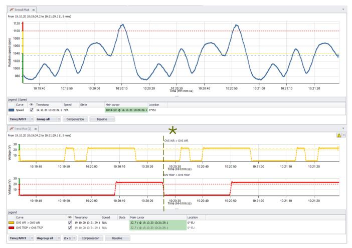
RL#4 (OVS TRIP) remains open, until RESET condition (\*), because latched condition
